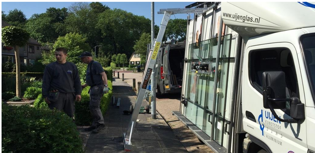
The Knight model M 2.4 to 4 meter with distance holder placed against a truck or A frame.
