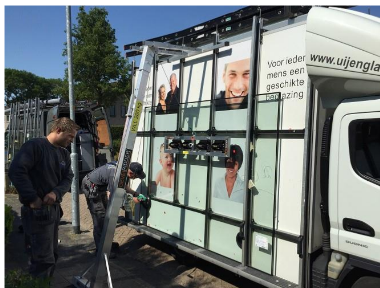
The Knight model M against the truck or A frame.
