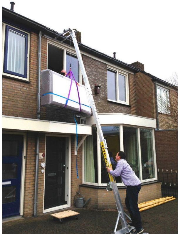
Model M with extra 3e piece up to 5.85 meter.
